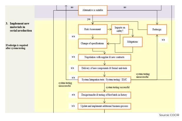
Figure 12: Flowchart step 3: Implementation in serial production.
