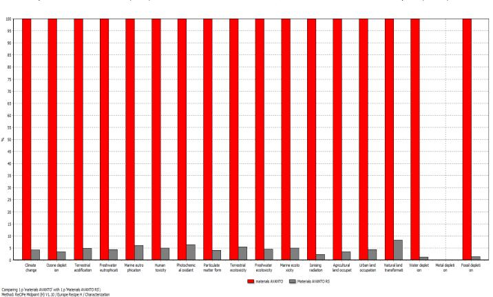
Fig 7 below shows the results of a Life Cycle Analysis assessment on the manufacturing of a MRI. This compares the impacts of a new device (RED) and those of a refurbished one, which includes 800 km transport (GREY).
